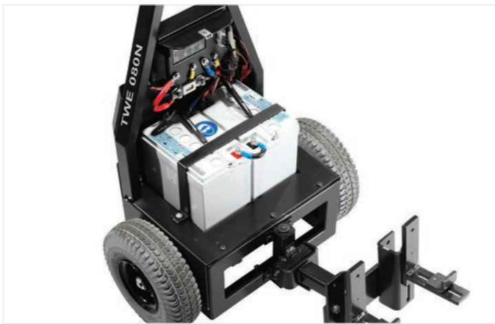
Maintenance-free gel batteries are fitted standard on the TWE080N.
