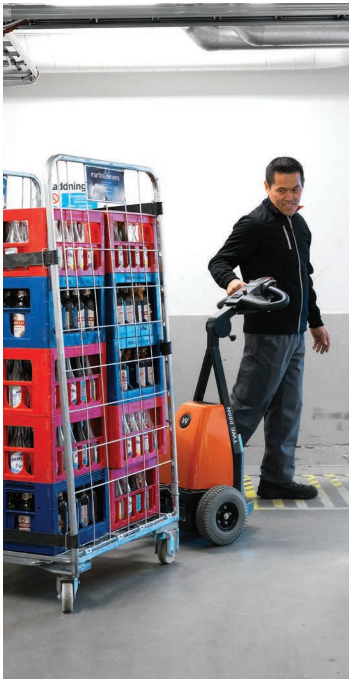
Control handle is comfortable and easy to use with a clear and concise battery status display.
