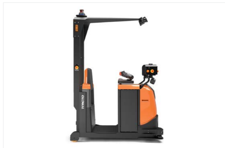
Automated tow trucks (Autopilot TAE500) can take over repetitive work between production lines & storage areas or conveyor systems.
