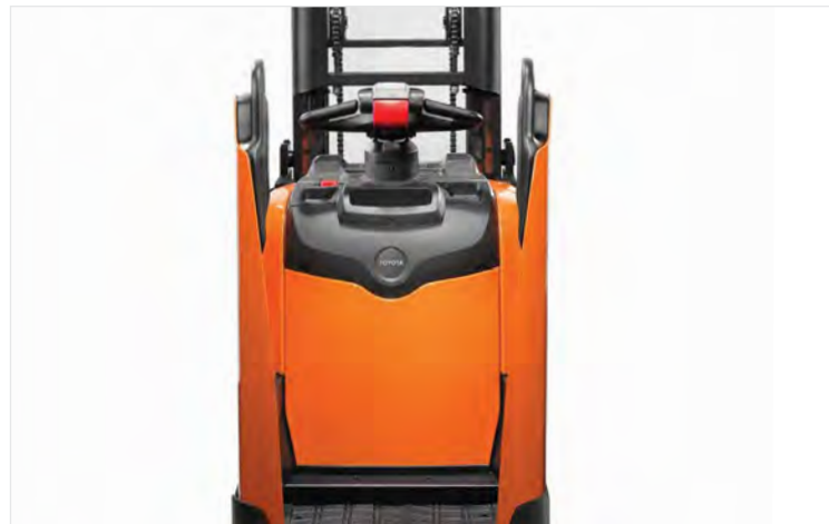
Side guards and E-man steering for comfortable and safe long distance driving
