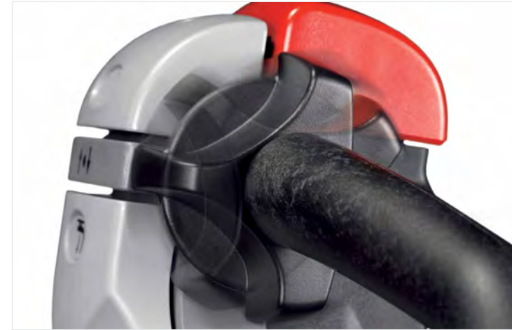
Ergonomic control handle, with emergency safety reverse button which, to avoid trapping, briefly reverses the truck if depressed
