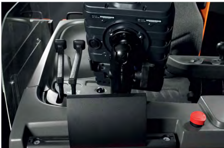
The E-bar universal mount for warehouse management devices such as PC terminals and barcode scanners
