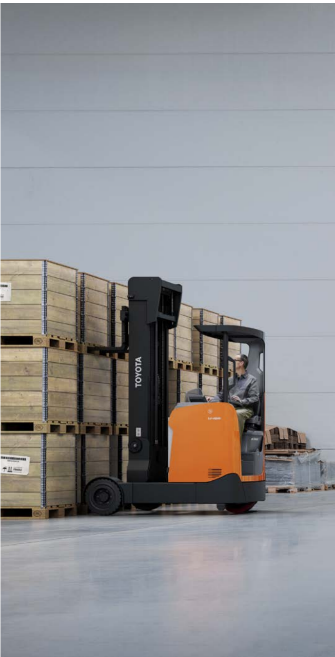
The BT Reflex O-series can handle road gradient and transition lines thanks to soft and elastic tyres, a durable drive wheel made from Redthane, and 145 mm ground clearance.
