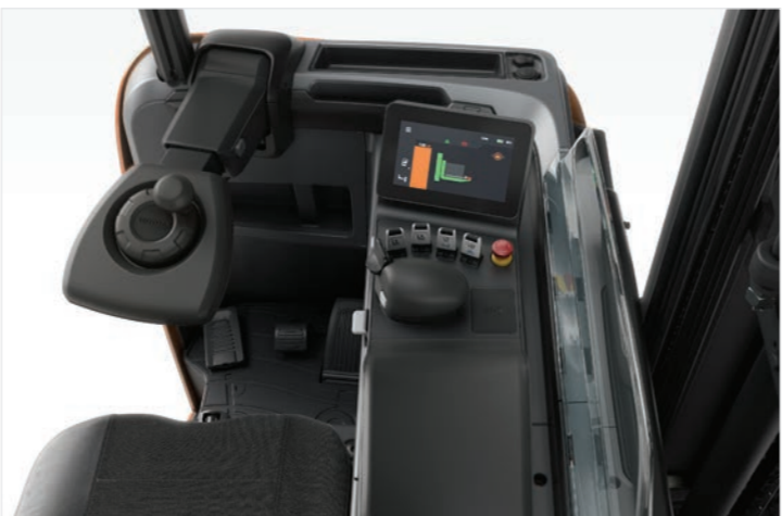
The operator compartment offers many different storage as well as dedicated space for PC with power outlet and a USB connector.
